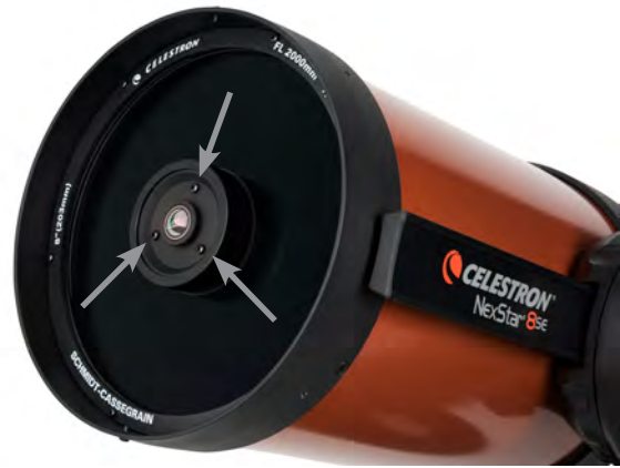
Secondary Mirror Collimation Adjustment Screws
