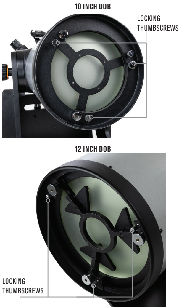
Figure 21: For the 10" and 12" Dobs, there are three spring-loaded collimation thumbscrews that adjust the tilt of the primary mirror. The other three thumbscrews lock the mirror in place once tilt adjustments are completed.
