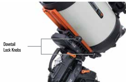
Figure 5 Telescope dovetail securely in place
